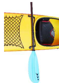
3 shaft-holder for reentry
