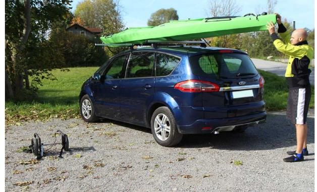
Now push the boat on the front of the roof rack and secure it properly with suitable lashing straps on the vehicle. The bracket is pushed back into the loading aid and secured.
